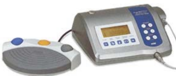
Specialised “driver” for the burr with controls for the surgeon to control the instruments direction of rotation, speed and torque..
